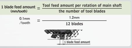
rotation of main shaft = the number of tool blades × 1 blade feed amount
